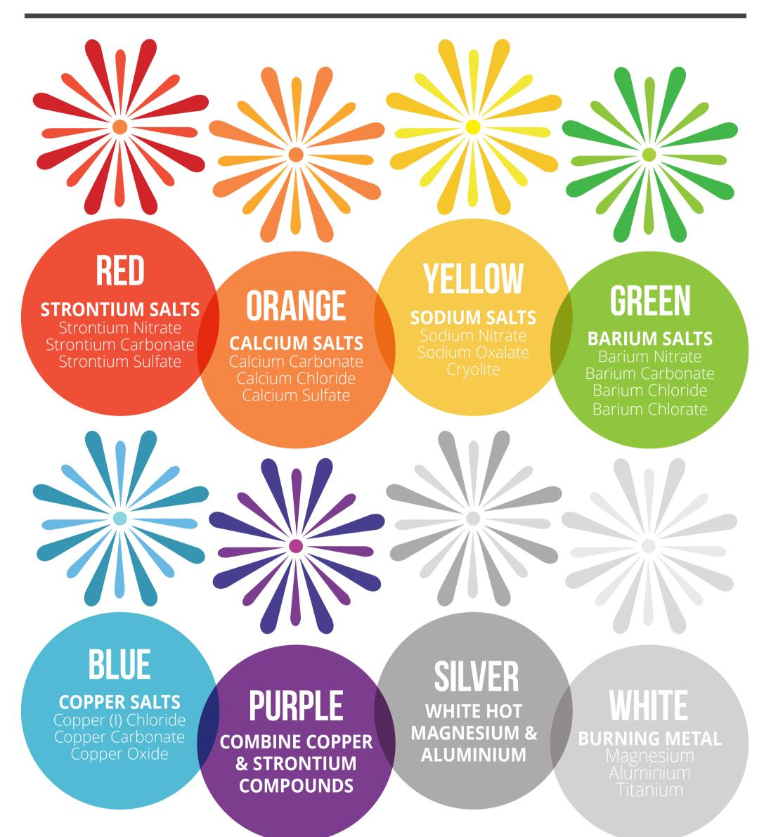
Colour in fireworks is produced by pyrotechnic 'stars', which produce coloured light when ignited. The stars contain five basic ingredients. **Metal salts** are used to produce colour; a **fuel** is needed to allow the star to burn; an **oxidising chemical** provides oxygen for the combustion of the fuel; a **chlorine-donating compound** helps strengthen some colours; and a **binding chemical** holds the mixture together.
